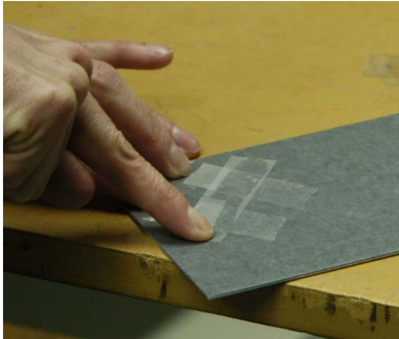
Applying more cellophane tape perpendicularly across the Mylar
